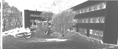
(h) Outdoor scene captured by the SWAP platform in 30 s (left) and captured by the FARO Focus 3D X 130 in 54 s (right) as a comparison.
