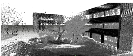
(h) Outdoor scene captured by the SWAP platform in 30 s (left) and captured by the FARO Focus 3D X 130 in 54 s (right) as a comparison.
